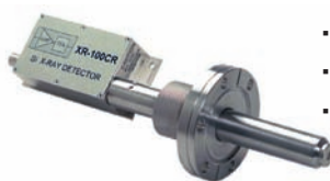
XR100CR fitted for vacuum applications
