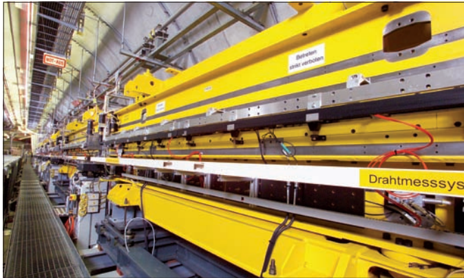
The 30 m-long undulator of the FLASH free-electron laser at DESY, the only such facility to produce high-intensity, ultrashort radiation pulses in the vacuum ultraviolet and soft X-ray wavelength range down to 6.5 nm. (Courtesy Manfred Schulze-Alex, Hamburg.)
