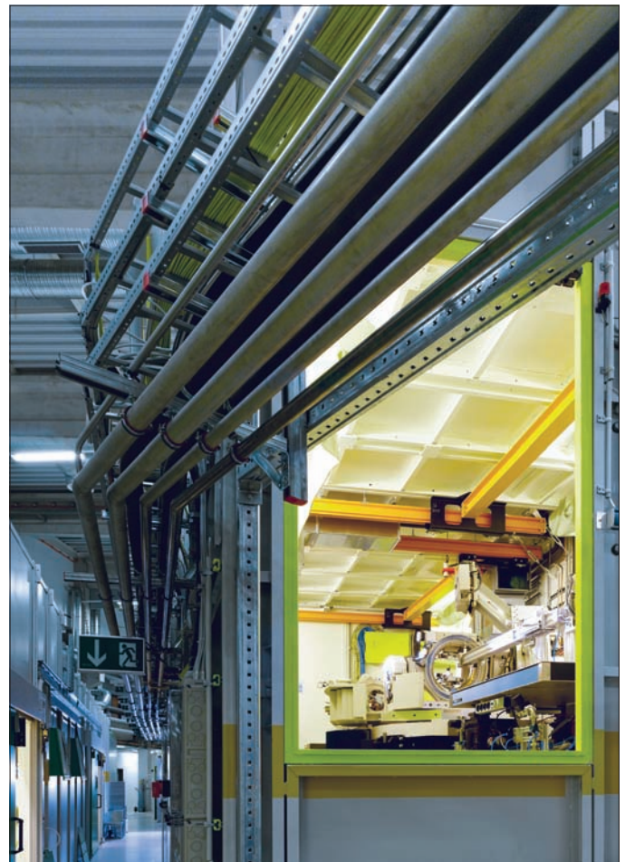
Measuring station in the experimental hall of the new PETRA III synchrotron radiation source at DESY – one of the most brilliant storage-ring-based X-ray sources in the world. (Courtesy Dominik Reipka, Hamburg.)
